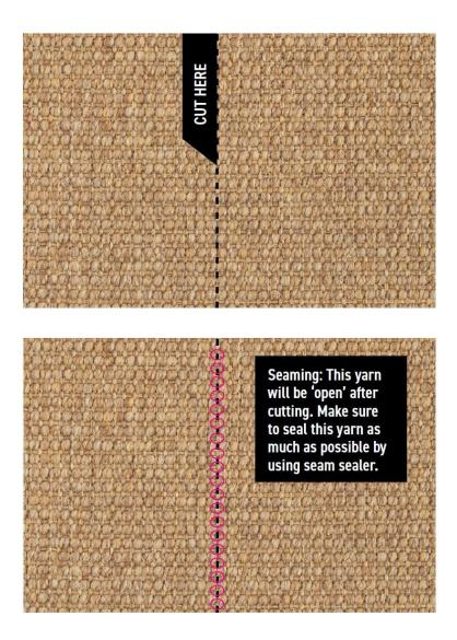
**Figure 1**: Cut 3rd row in from the center seam.
