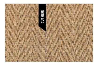
**Figure 1**: Cut 3rd row in from the center seam.
