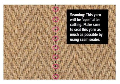
**Figure 2**: Take care to leave the lower lockstitch on the "good" side of the seam.
